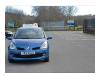
3) Counting the lines, starting with the right hand line of the bay you want to reverse into, count 3 lines when the 3rd line comes into the corner of the door and STOP. Apply the hand brake and select neutral.
