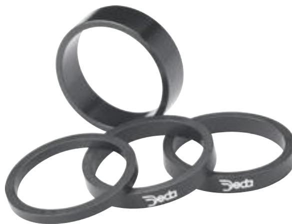
SPESSORI IN ALLUMINIO 6061 PER SERIE STERZO 1 1/8" CON FORCELLA CON CANNOTTO Ø 28,6 MM. SPESSORI CON DIAMETRO ESTERNO Ø 34,0 MM; Ø INTERNO 28,9 MM. DISPONIBILI ANODIZZATI NERI OPACHI IN ALTEZZA 3-5-10 MM.
