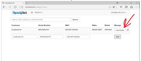
Step 7. After clicking "View Router" a modal screen will pop up that allows you to manage the router remotely. Click the "x" at the top of the screen to close the modal screen and add/manage another router.
