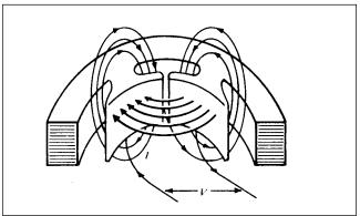
In the completed stator, a magnetic field is created having alternating north and south poles. The number of magnetic poles in the stator, together with the AC line frequency, determines the speed at which the motor will operate.
