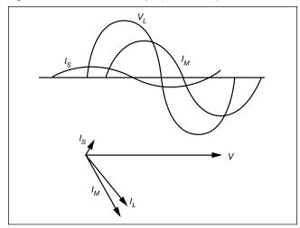
However, the real strength of the permanently split capacitor design is derived from the fact that the start winding and capacitor remain in the circuit at all times and produce an approximation of two-phase operation at the rated load point. This results in better efficiency, better power factor, and lower 120 Hz torque pulsations than in equivalent capacitor-start and split-phase designs.
