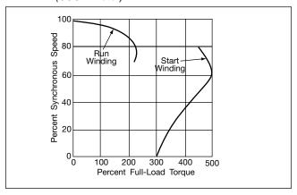
Table 4. Summary Capacitor Start-Capacitor Run Motor Characteristics
