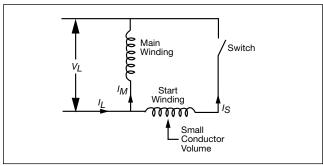
The main (run) winding is designed for operation from 75% synchronous speed and above. The main winding design is such that the current lags behind the line voltage because the coils embedded in the steel stator naturally build up a strong magnetic field which slows the buildup of current in the winding. This relationship between the line voltage and line current is shown in Figure 13.
