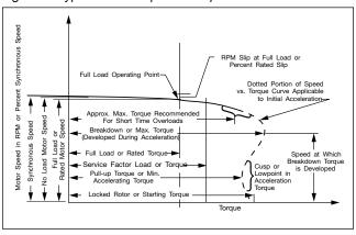
There are many torques that can be obtained from a motor's speed-torque curve:
