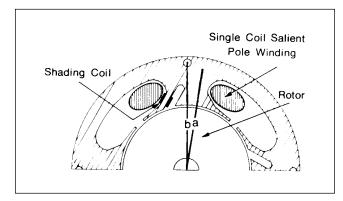
Figure 23. Shaded Pole Motor Construction
