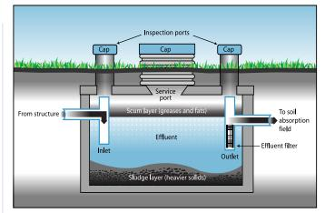
*Figure 2.* This diagram of a septic tank shows the three layers of waste: scum, effluent, and sludge.
