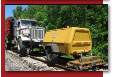
The Hulcher air evacuation service is an excellent fit for work around the hump yard, railroad signals and on the right-of-way. Air excavation cleans retarders, switches and crossings, loosening mud and fouled ballast quickly and cost effectively. It is also an excellent solution for exposing underground utilities. Air excavation works perfectly with a Hulcher hi-rail vacuum truck, which collects the loosened debris for reuse or disposal.
