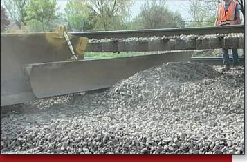
he Hulcher dozer rake service is a powerful yet economical solution that combines a standard Caterpillar® D5 dozer with a special, patent-pending rake attachment designed specifically for the even distribution or removal of ballast from beneath railroad tracks.
