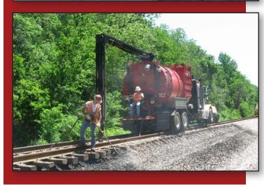
ulcher Services' Guzzler® Hi-Rail Vacuum Truck is a boom-equipped vehicle that uses vacuum power to pick up materials, which are stored in a collection tank for disposal or reuse. Unlike other trucks which are configured solely for track use, Hulcher's vacuum truck converts from road-ready to rail-ready in minutes to work in either setting.
