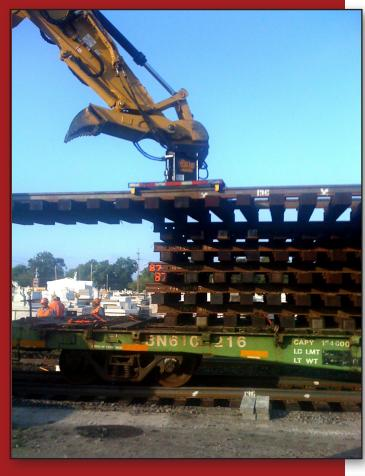
he Panel Boss<sup>®</sup> is an exciting system that revolutionizes the process of lifting, transporting and positioning rail track panel.
