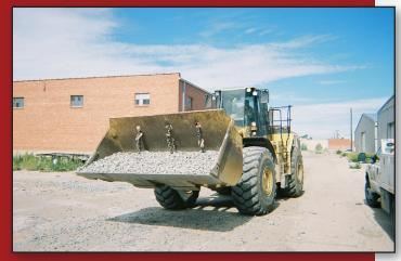
Hulcher Services' 980G wheel loader has an 11' 4" bucket with a capacity of up to 6.8 cubic yards, and can move and load large quantities of rocks, dirt or other materials quickly and effectively. An optional fork attachment increases the 980G's capabilities.
