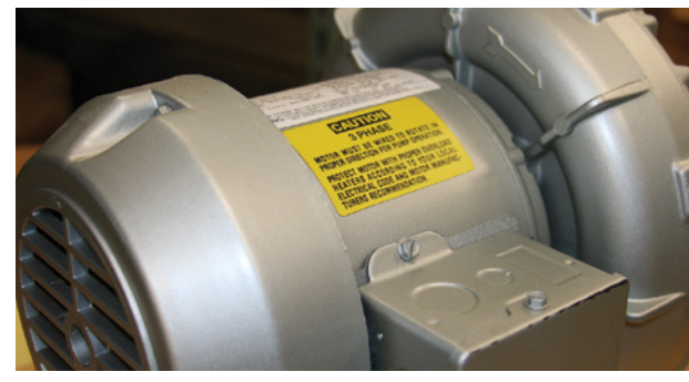
Overlamination will protect against abrasion, some solvents, oil, gasoline and some acids.
