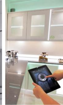
The 4 zone remote control system allows the user to control four different lighting circuits from one remote control without the need to physically wire them together. It allows you to switch up to four different areas on, off or dim at the same time, or individually.
