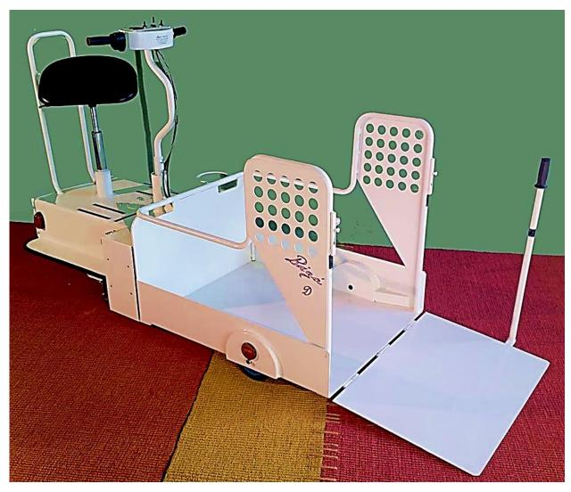
Electric lawn tractor that allows an operator to load on the loader trailer any trolley effortlessly as the cargo floor is only 6 cm tall with a climb ramp less than 5%. Closing the flip takes place quickly and without burdening the operator back, given the ergonomic handle. The size is are such as to allow the entry and exit of Bigà type D lawn tractor in very limited spaces such as lifts with depth of 200 cm. The rear driving-wheel
