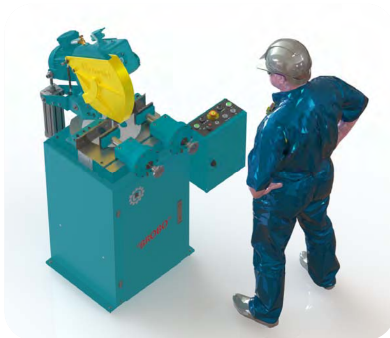
Figure 6. Correct Position for Operating Saw Unit
