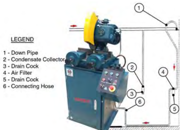
Figure 5. Ideal Air Supply Connection
