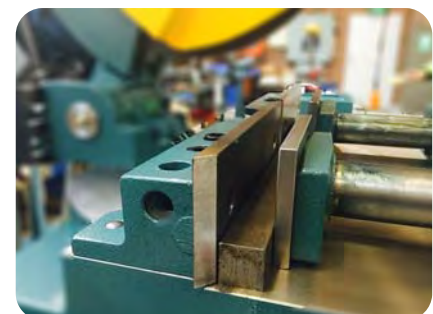
Figure 16. Clamp Clearance 3-7mm
