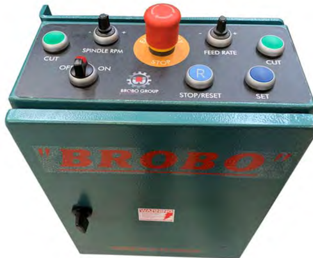
Figure 12. PLC Control Box
