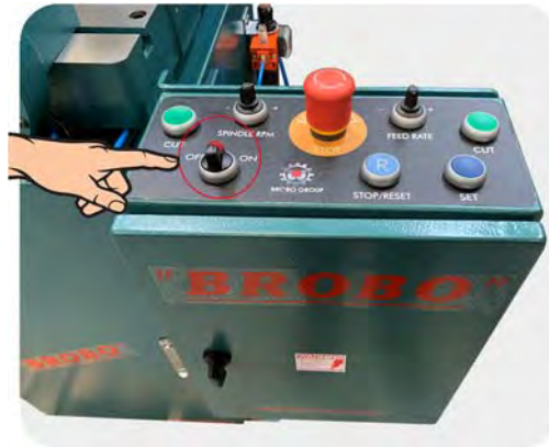
Figure 4. Main Control Switch
