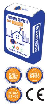
PREMIXED PLASTER BASED ON NATURAL LIME AND CEMENT FOR BASE COAT PLASTER TYPE "FR" FIBER REINFORCED – "I" WATER REPELLENT FOR STRUCTURAL USES CLASS R1-CC Compliant with UNI EN 998-1 UNI EN 998-2- UNI EN 1504-3
