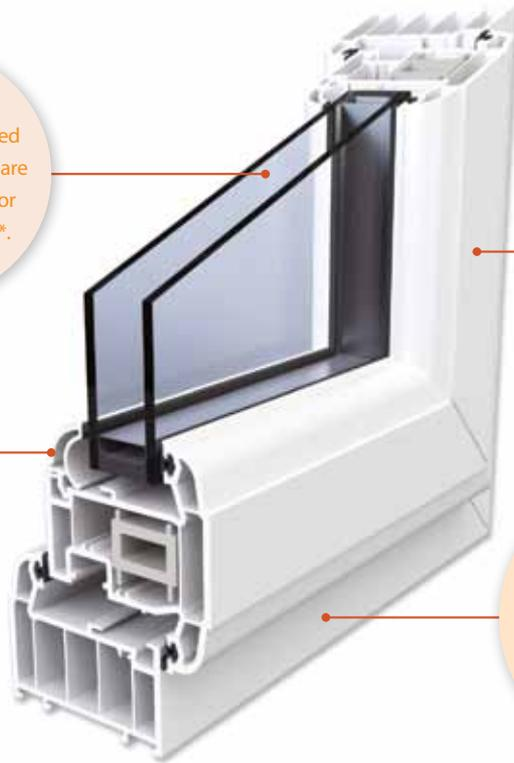
Opening frames are fully weather-stripped and reinforced with 100% recycled PVC-U bars for added strength and increased thermal performance.
