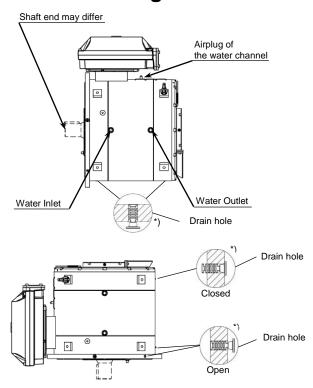
Figure 1. Connection of cooling water, air plug and condensation drain holes. \*) IP65 drain holes plugged with M6 screws.
