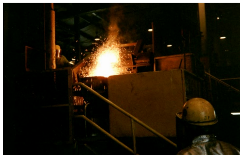
Fig 7 A four tonne iron powder atomiser
