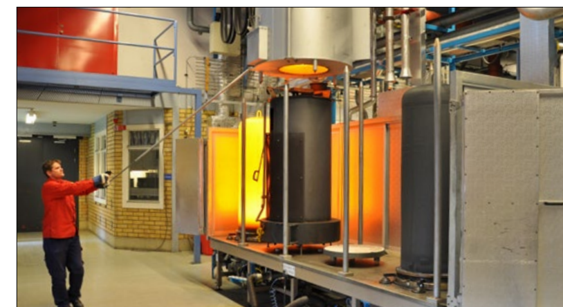
Fig. 7 Hot wall vacuum retorts used for high temperature CVD coating. One heating unit serves several process retorts
