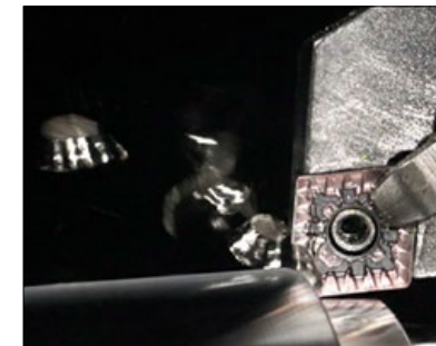
The WIDIA Victory turning portfolio features the Universal Roughing geometry for smooth chip forming
