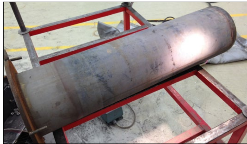
Fig. 8 Vacuum sintering retort made from Kanthal APMT used for five months at approximately 1250°C temperature
