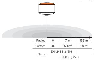
How to read the drawing : In a range of 15.5 meters, being a surface of 750  $\,\mathrm{m^2}$ , we guarantee a lighting in accordance with the standard EN1838
