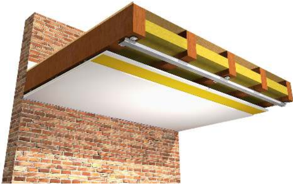
Timber Joist Ceiling
