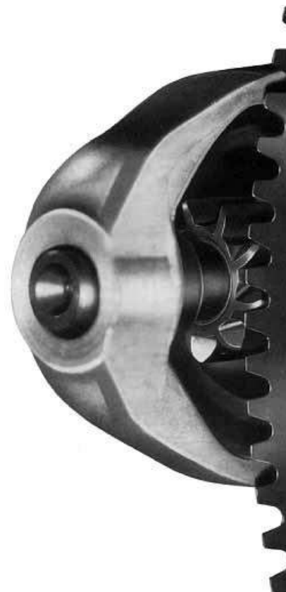
Starter pinion (small gear) fully meshed with the ring gear of engine flywheel (large gear).
