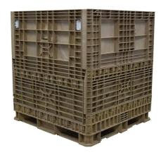
The 45 x 48 x 50 hopper bottom container, with its smooth, funnel-shaped interior, is ideal for controlled dispensing of seed, grain, resins, powders, pellets, and other small components. The hopper empties contents in about 30 seconds. Made from high-density polyethylene, this 2,000 lb.-capacity, collapsible bulk container will provide years of reliable service under the toughest conditions. 100% recyclable. Optional black lid. Beige color.
