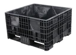
The Ropak® 30 x 32 x 18 fixed-wall bulk container is a shorter, sturdier container with non-collapsible side walls and a single-piece molded base. With a 2,000 lb.-capacity, the reusable container is ideal for applications with high-weight and low-volume requirements. 100% recyclable. Optional lid.
