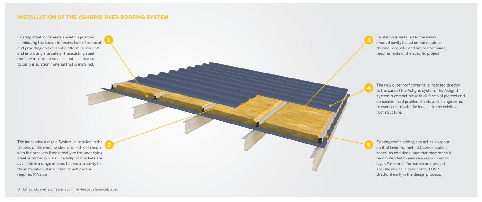
2 Ashgrid Over-Roofing Spacer System
