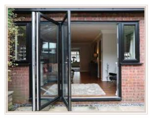
Bi-folding doors can open internally or externally. Either way, panes fold flat against each other and sit neatly out of the way.
