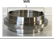
To identify the size of fitting measure O.D. of the buttweld stem.
