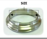
To identify the size of fitting measure O.D. of the buttweld stem.
