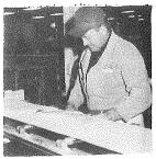
on the fish stick line, making sticks out of haddock, cod and pollock. The fish is chopped into stick size and goes through batter and breading machine. From here the sticks go into a cooling room, until their
