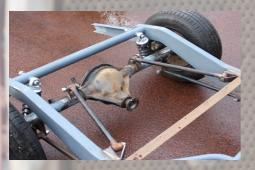
These four bar systems are ideal for cars that have wide chassis rails with a kick up on the rear over the diff, typical of 1932 onwards. They are a simple four bar system that dose not require a panard bar, and allow the car to sit at a nice ride height. This one is fitted to one of our standard 1928 combo chassis, under a 1928 Ford Closed Cab Pickup
