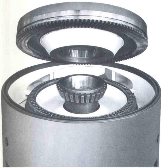
Spindle Bearing — 36" Dynatrol V.T.L.
