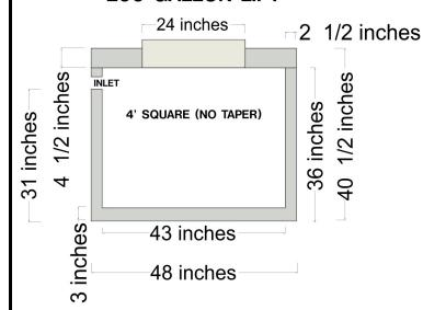
REGISTERED IN MINNESOTA FOR SEVEN FEET OF COVER ON TOP OF THE TANK.
