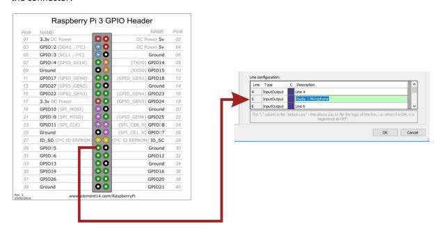
The diagram above shows how GPIO Line 5 on the Pi (physical pin 29) is directly linked to Virtual Line 5 in the hardware service, so if you trigger an input on GPIO Line 5 on the Pi, Virtual Line 5 will automatically reflect that in the Hardware Service.
