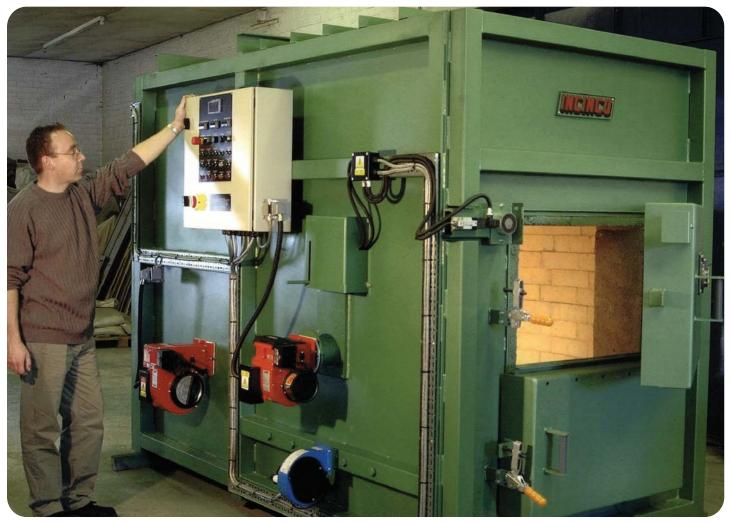
Free standing unit requires a flat surface. Modular package type with Primary and Secondary chambers, designed to give a residence time of 2 seconds up to 1000 to 1200°C. Based on Pyrolytec Combustion Principle.
