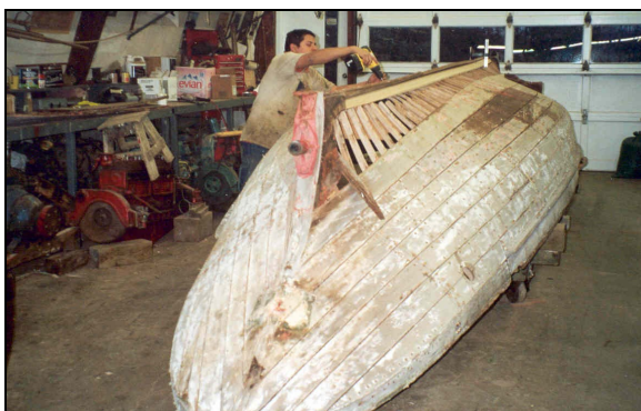
New keel installed – original cypress planks were checked and reinstalled
