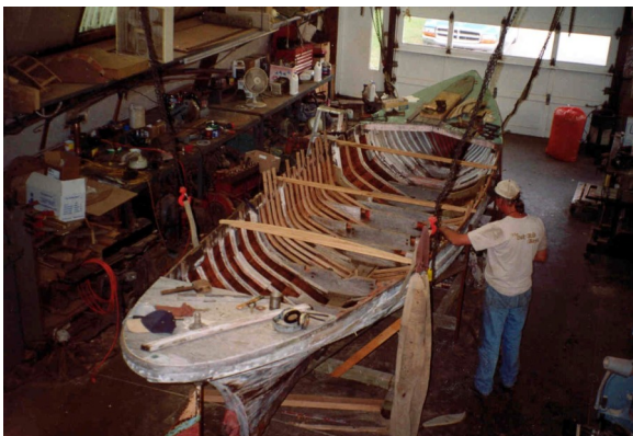
New ribs installed
