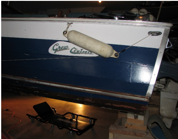
Muskoka bumper system. Pull chord from front seat and it raises all 3 on each side
