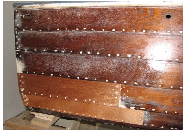
Close up of new planks and filled holes
