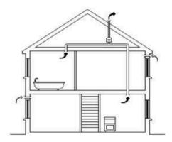
An MVHR system comprises a central MVHR unit connected to an air distribution system. A fan in the MVHR unit gently removes stale, humid air from wet rooms (e.g. bathrooms, kitchens, cloakrooms) and expels it to atmosphere.
