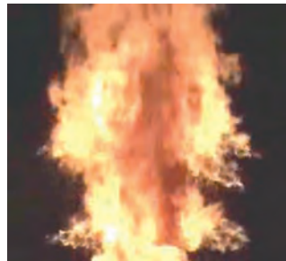
Step 3: The manikin is exposed to flame engulfment for four seconds.
