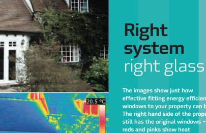
effective fitting energy efficient windows to your property can be The right hand side of the property still has the original windows - the reds and pinks show heat escaping. However, the new extension on the left is fitted with energy efficient windows, the lack of reds and pinks proving they help dramatically reduce heat loss
