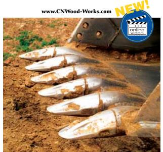
Komatsu's KMAX tooth system offers durability in more than 20 tooth styles for a wide range of excavators and wheel loaders. It's easy and safe because the system requires only a socket wrench — no pins to hammer — to remove and replace teeth from the adaptors.
