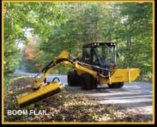
The Trackless Series MT 6 features a 110 hp Tier 3 Cummins diesel, joystick control for attachment functions and an electronically controlled hydrostatic system which is linked to the engine rpm. The cab and rear chassis have been re-designed and includes several technological, ergonomic and performance related advancements over the previous Series MT5
