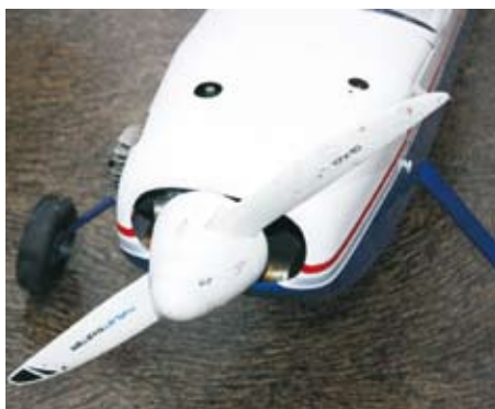
Openings for the needle valve and onboard glow igniter. Ample cooling with small flap underneath
