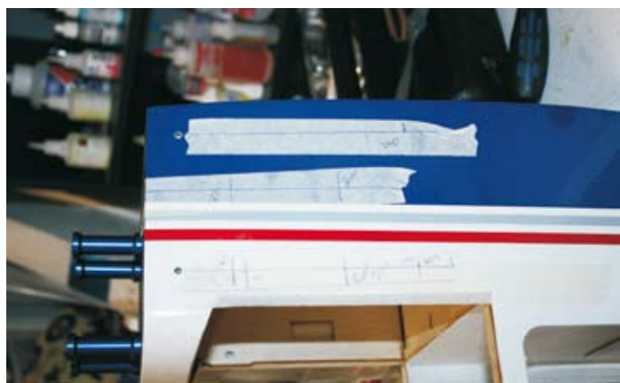
Purely for convenience, the supplied engine mount standoffs substituted for OS M5 units
