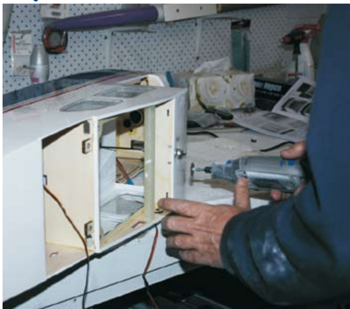
Trim the pushrod release wire after setting ATV
