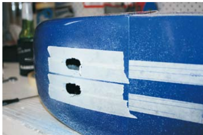
Masking for the Bisson Pitts muffler outlets, OS 160 FX
