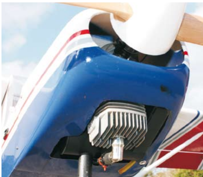
Side mounted OS 160FX OS GT 33 inverted installation
