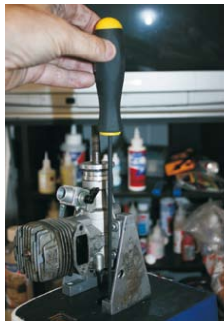
Dubro ball tip driver dipped in white out marks where to drill
