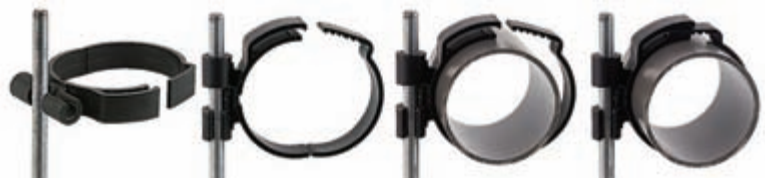
Slide onto threaded rod, twist to engage Insert pipe and clip to lock
