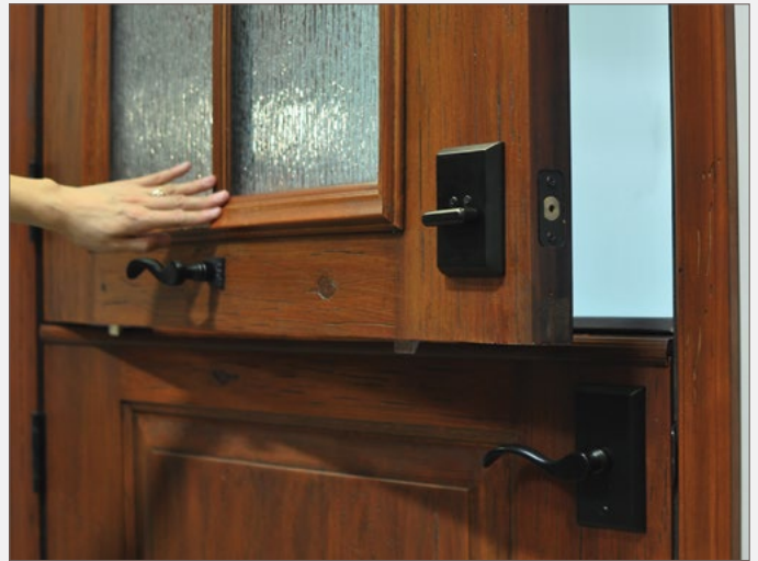
This view of a partially open Dutch Door shows the kerfed astragal and the Q-Lon weather seal used to prevent energy loss, reduce noise, light, and dust, and seal from precipitation. The bottom rail of the top half — and the top rail of the bottom half — are constructed using a no-rot composite material. This photo includes our Multipoint Lever Latch option.
