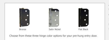
All pre-hung units use 3 ball-bearing hinges on 6'-8" tall doors and 4 hinges on 8'-0" tall doors. 1-3/4" thick doors use 4 inch hinges, while 2-1/4" thick doors use 5" hinges. Choose from these three hinge color options shown at left for your pre-hung entry door unit: Bronze, Satin Nickel or Flat Black.
