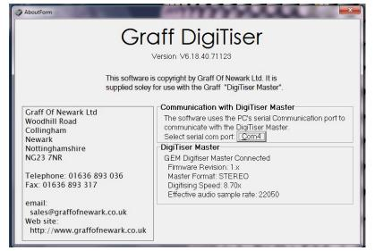
From here you can select the com port that the Digitizer is using. Select each one in turn until you see the information about the Digitizer displayed in the box below the com port selector. The sound cards will be automatically assigned on exit from this page. Mono users are now set up and ready to go.
