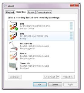
Select the 'Recording' tab at the top. A double click on the 'BEHRINGER UMC 20xHD 192k' will bring up the 'Properties' window. Click on the 'Advanced' tab and select the sample rate of '2 channel, 24 bit, 192000 Hz, (Studio quality)'. Click 'Apply' then 'OK' and close both windows. Stereo users repeat for the other sound card too.
