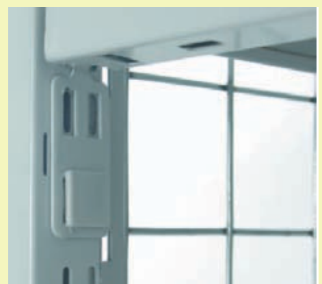
This unique clip simply slots into an upright and is secured with a plastic fitting so that shelves cannot be dislodged accidentally.
