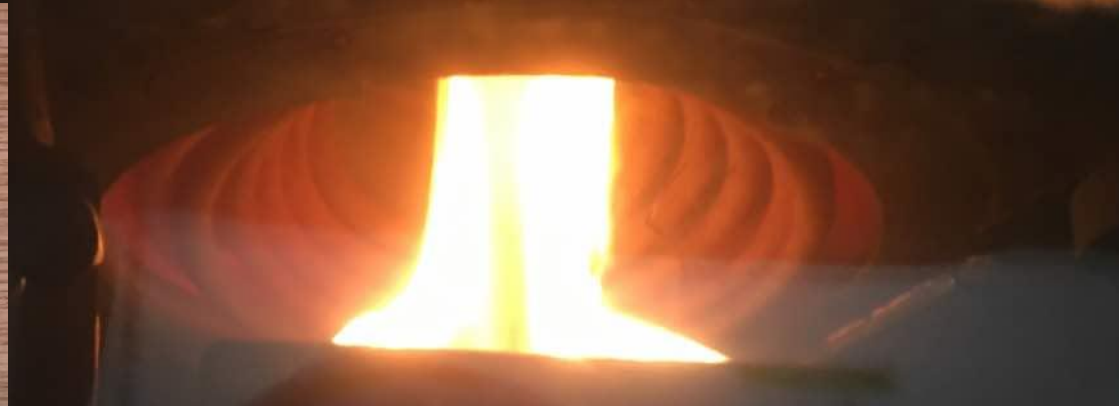
Biomass flame through observation window
