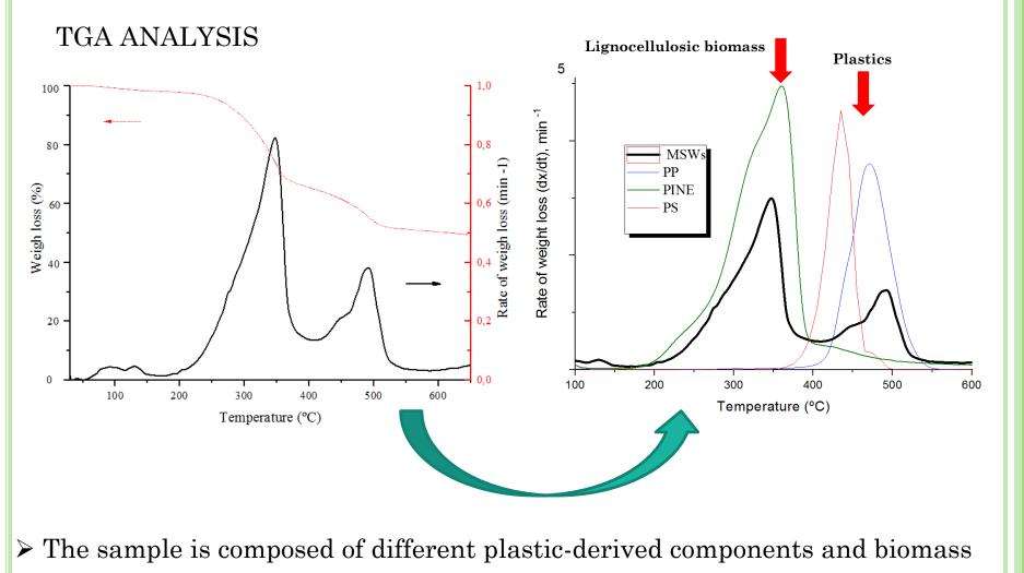
> 550 °C seems to be sufficient temperature to carry out the devolatilisation of this particular MSWs to complete its total conversion
