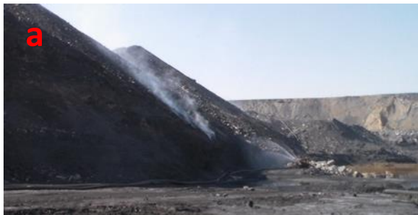
Figure 1: (a) Self-heating of run-of-mine (b) Aerial View of stock pile of coal discard at Mpumalanga Highveld, South Africa (c) Slurry dump, adjacent to a coarse discard coal dump
