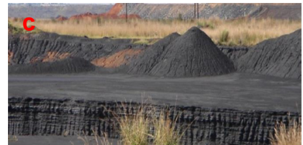
Figure 1: (a) Self-heating of run-of-mine (b) Aerial View of stock pile of coal discard at Mpumalanga Highveld, South Africa (c) Slurry dump, adjacent to a coarse discard coal dump
