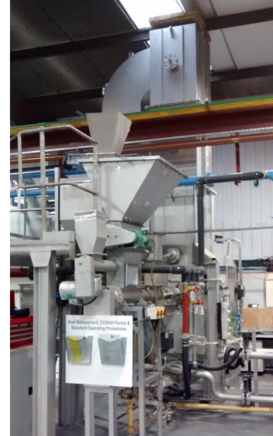
Above: Pilot-scale fluidized bed combustor used.
