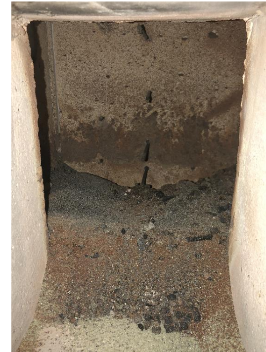
Left: Image of 664 \mu m olivine bed material prior to use. Right: Bed condition after wheat straw/olivine test.
