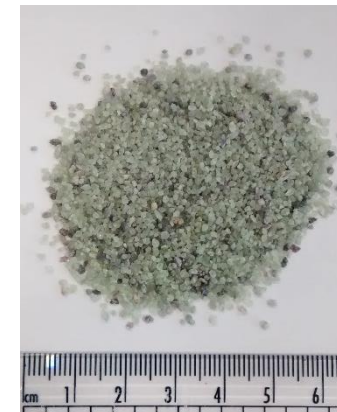
Left: Image of 664 \mu m olivine bed material prior to use. Right: Bed condition after wheat straw/olivine test.
