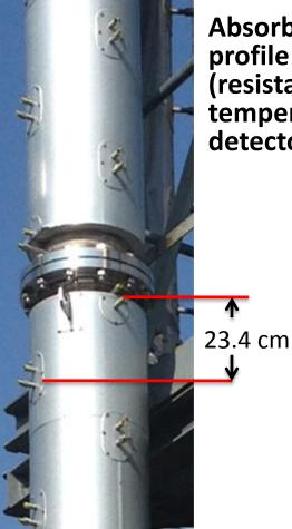
Absorber temperature profile by ten RTDS (resistance temperature detectors)
