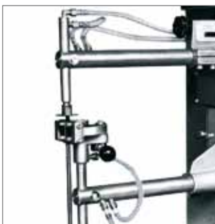
VICE ELECTRODE for welding of one sheet disc on one rod. The rod carry the current and is clamped in a vice electrode.
