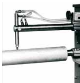
ROD ARM for spot welding of cylindrical parts. The fitting is infinitely adjustable from 130-500 mm.
